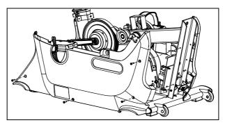
Figure 4: Side cover removal
